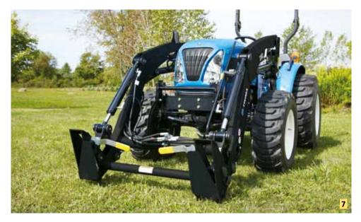
4 | Modern and high performance style. Smart and performanceenhancing design is typical Trima. One example of this is the smooth-curved loader beam which matches the curve of the tractor's bonnet. Another example is the robust and strong bearing box, which provides an optimal line of sight thanks to its slim design.
