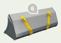
**6.** The implement hooks contribute to the strong design. You will notice that hooks and locking holes are positioned along a fold in the metal. Depending on bucket model and size, there may be a double profile sheet inside the bucket.
